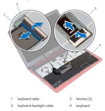
**5** Lift the keyboard, along with the cables, off the palm-rest assembly.
